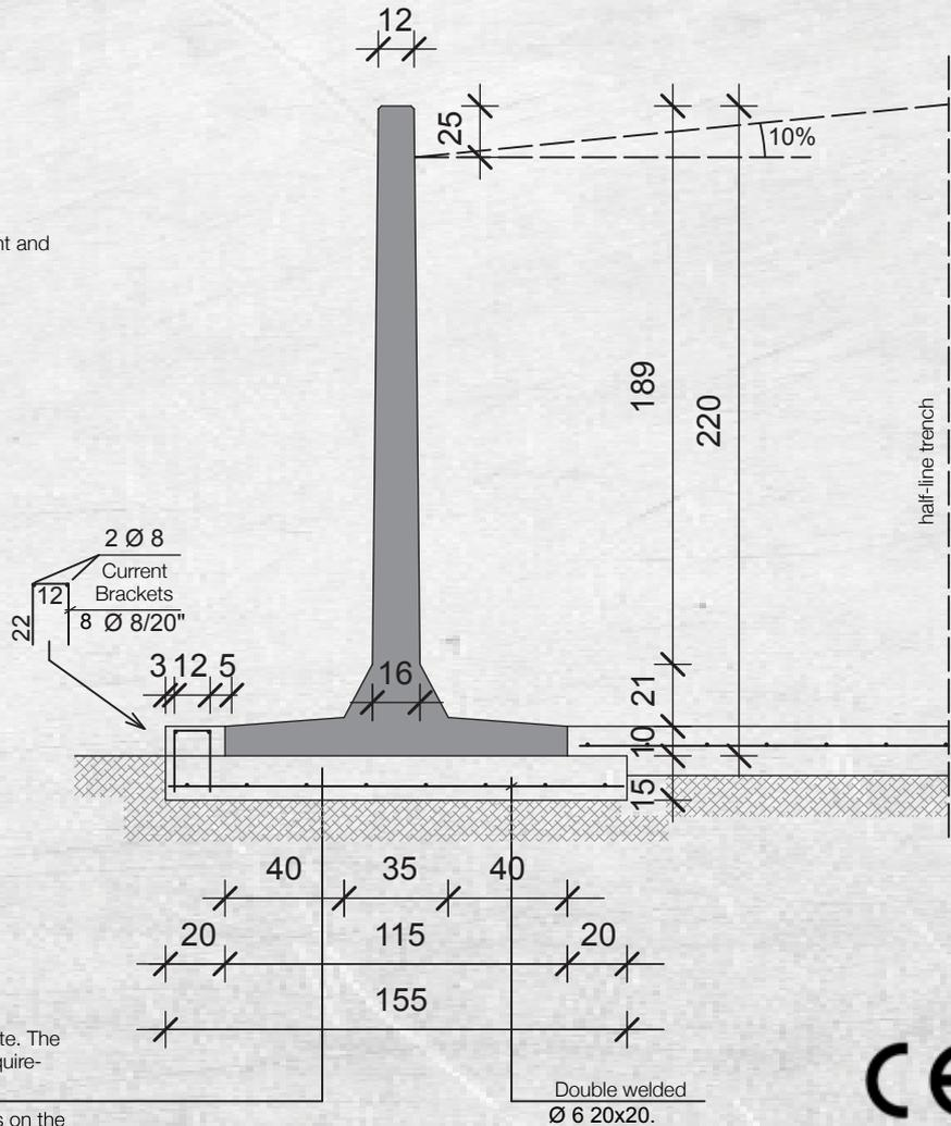
Concrete foundation to be carried out on site. The thickness is 15 cm for the land capacity requirements as indicated in the table.
