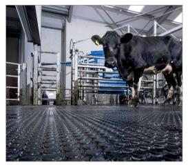
EASYFIX MG Max 8 has a high grip penny type surface and is ideal for use in areas of high traffic, on large farms.
